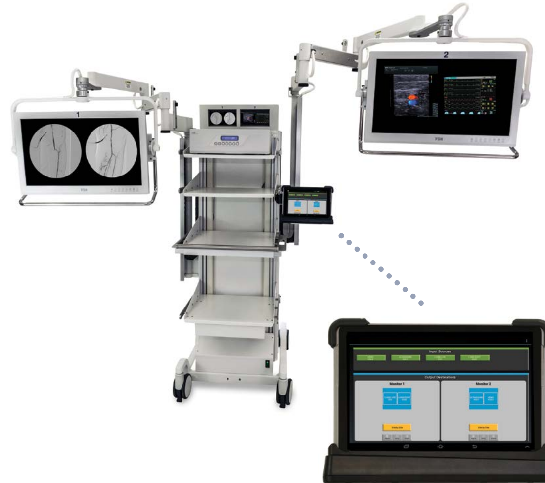
Intuitive tablet control of image routing
