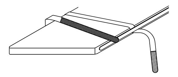
SLIDE THE RESTRAINT STRAPS OVER THE TABLETOP AND THROUGH THE SPACES BETWEEN THE ACCESSORY RAILS AND THE TABLETOP.
