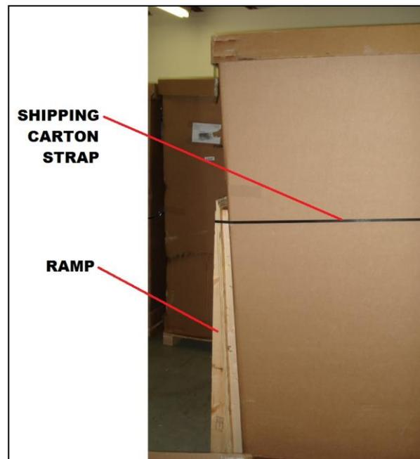
Step 5. Remove the top part of the shipping carton which will allow the sides to fall away from the MDS cart.
