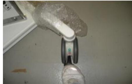
Step 11. Slowly roll the MDS cart off of the skid and down the ramp until it is completely off of the ramp.
