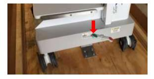
Step 10. Slowly roll the Ilex 55 cart off of the skid and down the ramp until it is completely off of the skid.
