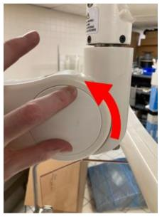
Remove the outer clam shell of the spring arm by removing the screws on each end of the spring arm. There will be one screw on each end of each long clam shell. (On the light head spring arm there will only be one side with screws, the other side slides into the end nearest the light head. Using a wide blade screwdriver pry the shell apart taking care not to damage the plastic. Save all parts for reinstallation later.
