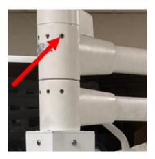
After the brake screws have been set, the rest of the unit should be checked to verify functionality. The central axis should be allowed to rotate 320 degrees with stops in the rear. The joint between the horizontal and spring arm should allow for 360-degree rotation. The radiation shield should be able to rotate 360 degrees about its axis, and the light should also be able to rotate 360 degrees about the axis joint. Lastly both spring arms should be able to be moved up and down vertically.
