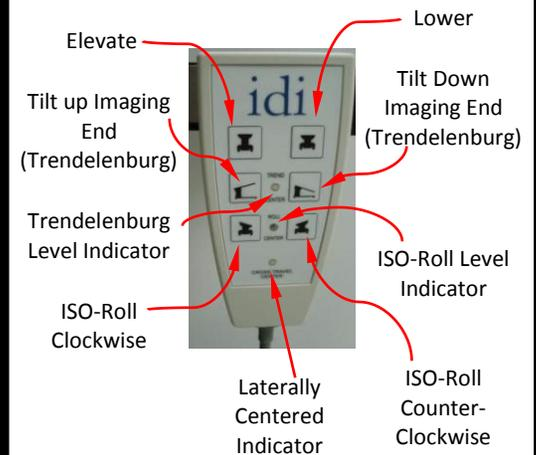
It is recommended that the pendant control be disconnected during critical procedures to prevent inadvertent operation or motion, causing patient injury. The Motion Lockout Pushbutton on the Panhandle Unit **does not** disable the Handset Control.
