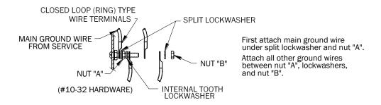
5. Connect all monitor ground wires and the service ground wire as shown in the figure above. (The number of wires varies with the number of monitors installed).
