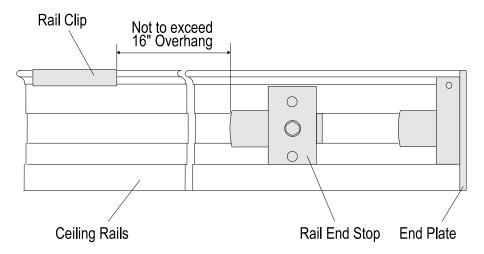
WARNING! The position of the Rail Stop must not exceed 16" rail overhang or damage to the system may result.
