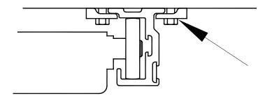
3. Check that the hardware securing the end plates are tight.
