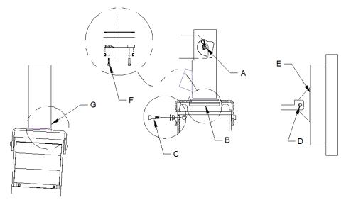
7. Check the pad attached to the underside of the monitor mount. If there is any damage to the pad or if the pad is not properly attached to the unit, it must be replaced.
