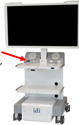
Ilex main power "ON/OFF" switch
