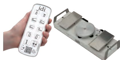
Wireless footswitch and pendant hand control
