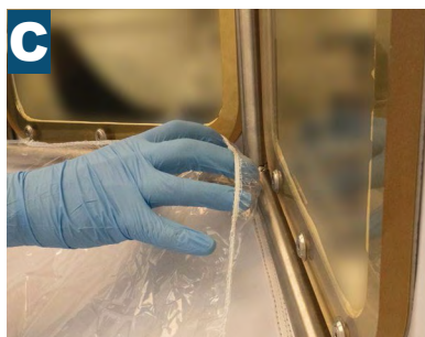
Place drape on hooks on head-side of Protego Shield
