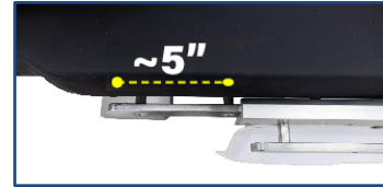
Leave at least 5" of rail exposed when adding Side Shield
