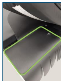
Lift left-side Armboard pad to find the removeable led section (outlined in Green in the image to make it easy to see).
