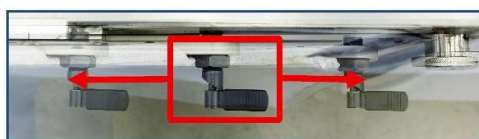
Center black lever facing PT feet to easily slide in both directions.
